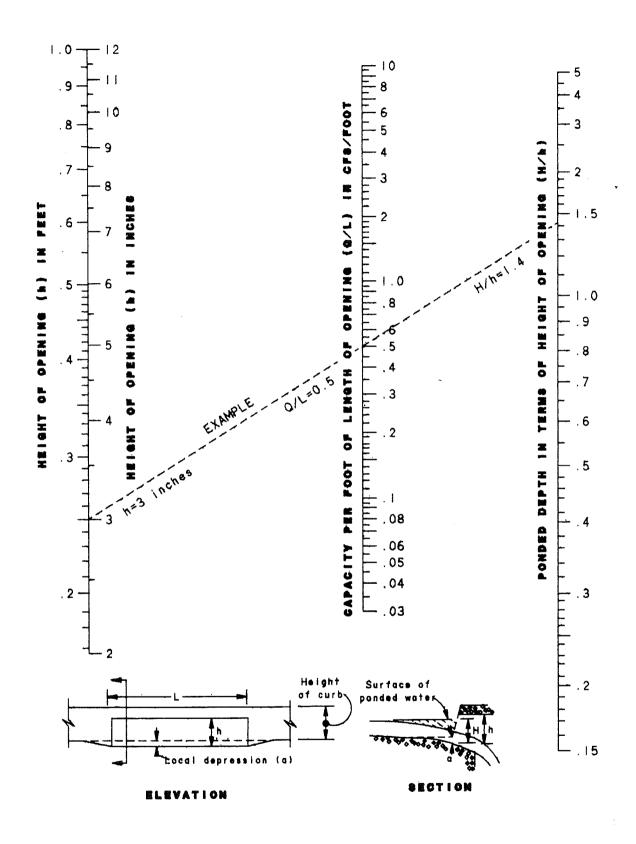
CAPACITY OF CURB OPENING INLET AT LOW POINT IN GRADE (STREET INTERSECTION)
