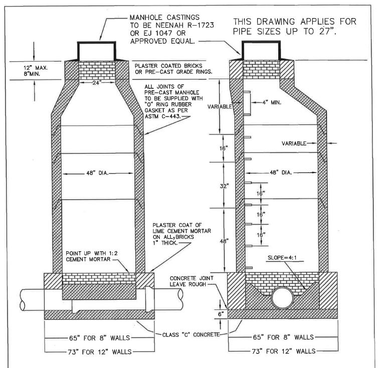
NOTE: ALL MANHOLES SHALL BE CONSTRUCTED TO THE ELEVATION OF THE PROPOSED STREET GRADE OR TO THE PRESENT GROUND ELEVATION, WHICHEVER IS HIGHER, UNLESS OTHERWISE ORDERED.
