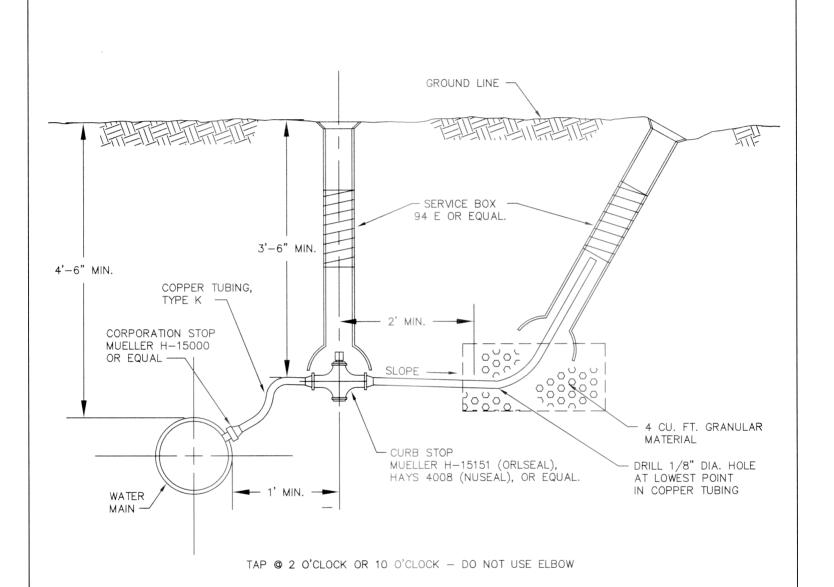
NOTE: THIS TYPE BLOW-OFF IS TO BE USED WHEN A FIRE HYDRANT IS NOT INSTALLED AT END OF LINE.
