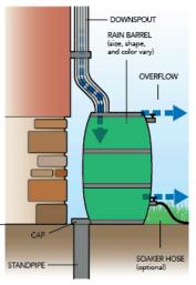
DOWNSPOUT CONNECTED TO RAIN BARREL
