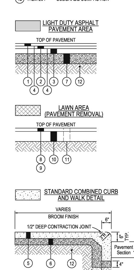
STANDARD CONCRETE WALK WHERE CURB IS NOT PRESENT SHALL MATCH THE BUILD-UP OF THIS DETAIL.
