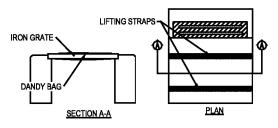
INSTALLATION: STAND GRATE ON END. PLACE DANDY BAG OVER GRATE. ROLL GRATE OVER SO THAT OPEN END IS UP. PULL UP SLACK. TUCK FLAP IN. BE SURE END OF GRATE IS COMPLETELY COVERED BY FLAP OR DANDY BAG WILL NOT FIT PROPERLY. HOLDING HANDLES, CAREFULLY PLACE DANDY BAG WITH GRATE INSERTED INTO CATCH BASIN FRAME SO THAT RED DOT ON THE TOP OF DANDY BAG IS VISIBLE.
